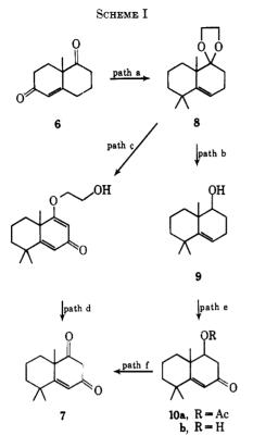
path a, HOCH<sub>2</sub>CH<sub>2</sub>OH, H<sup>+</sup>; CH<sub>3</sub>I, (CH<sub>3</sub>)<sub>3</sub>CO<sup>-</sup>K<sup>+</sup>; NH<sub>2</sub>NH<sub>2</sub>,
